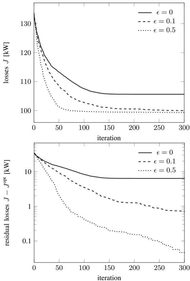
Fig. 3. Montecarlo analysis of the behavior of the algorithm for different values of  $\epsilon$ . As soon as  $\epsilon$  is greater than zero, the algorithm converges to the optimum. Also the rate of convergence depends on the choice of  $\epsilon$ . In this comparison we assume that one iteration corresponds to a complete iteration of the algorithm, regardless of how many hops are required for its completion.
