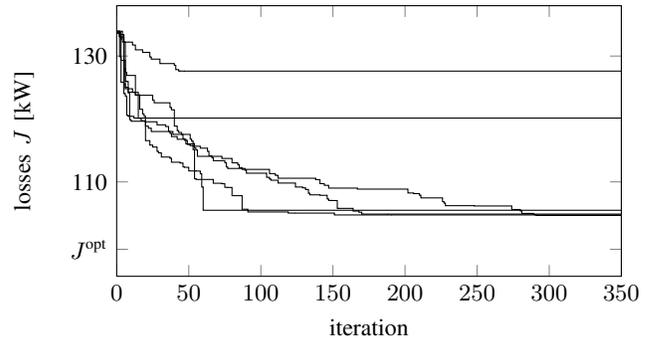
Fig. 2. Multiple instances of the algorithm when  $\epsilon = 0$ , i.e. there is no multi-hop strategy. Different randomly generated initial conditions correspond to different steady state configurations of the compensators, none of which results to be optimal.
