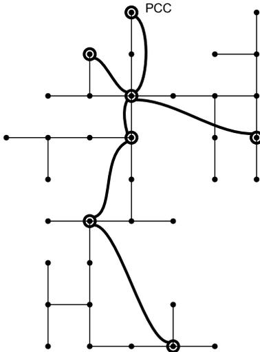
Fig. 1. The thin lines represent the graph  $\mathcal{G}$ , which describes the electrical topology of the micro-grid (in this case, an adaptation of the IEEE37 testbed). Circled nodes are compensators (belonging to  $\mathcal{C}$ , while the other nodes represent loads). The thick lines represent the edges of the communication graph  $\mathcal{H}$ , describing which compensators can communicate via PLC.
